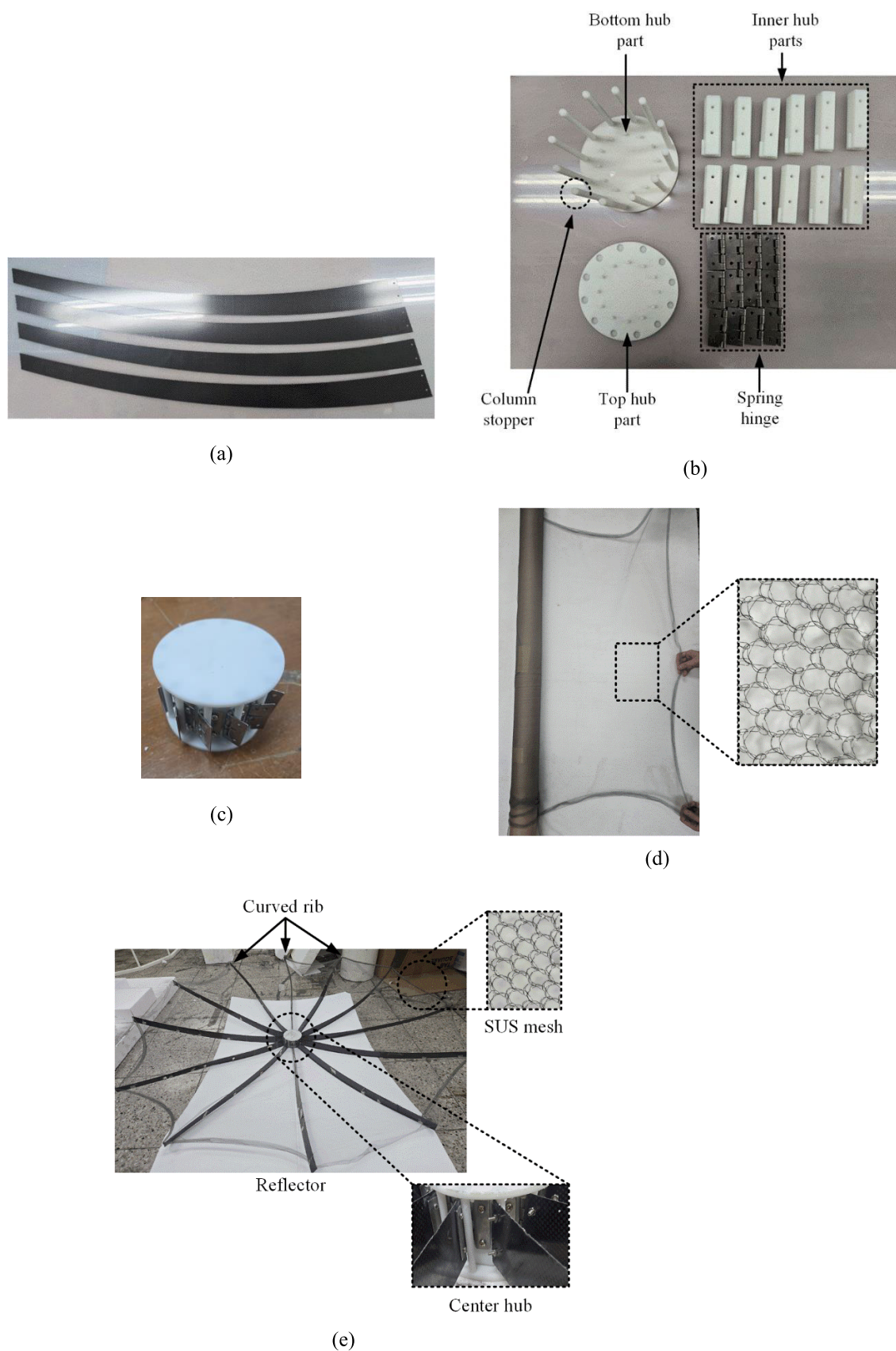
FIGURE 6. Photographs of the fabricated proposed antenna. (a) Curved ribs. (b) Each part of the center hub. (c) Fully assembled center hub. (d) SUS conducting mesh. (e) Fully assembled mesh reflector.
